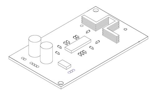
4. **High Voltage Supply (HVS) –** Green board with orange capacitors and black metal ridged object
