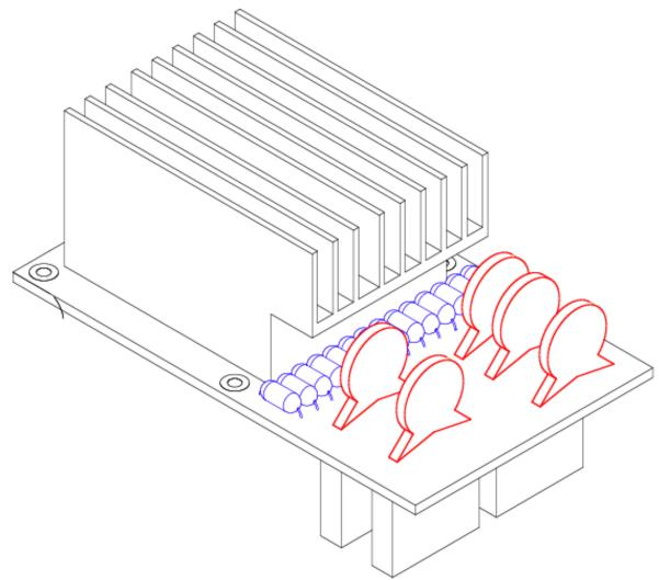
The high voltage pod requires other voltage to power it; it then amplifies that voltage and exports it through the cable connectors at its base. There are two options for providing a voltage to the HV pod. First, it is possible that CROP has a low voltage power supply strictly for this use (we did in my days). This is the easiest method.
